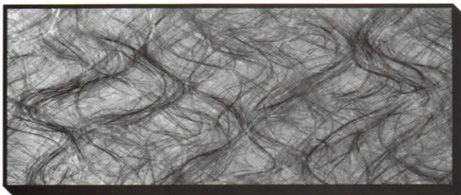
Fiberglass fibers are sanitized and woven into a controlled density pattern.
