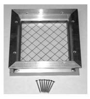
The Steril-Aire AHU Viewport provides a safe, effective means to view working UVC Emitters<sup>™</sup> inside an air handling unit (AHU). The AHU Viewport provides installation flexibility for AHU insulated walls of 2" (5.1 cm). It provides the ability to view the interior of the AHU through a 6" x 6" (15.2 cm x 15.2 cm) clear wire glass without the need to open access panels/doors or disconnecting circuits while offering personnel protection against exposure to UVC light.
